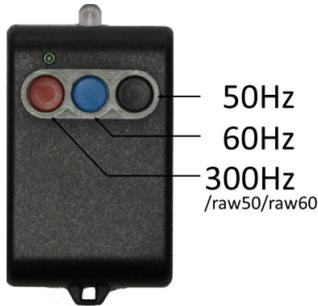
The right button is for "50Hz" platters and discs.
